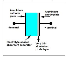
way, but the electrical connection to the other side of the oxide layer is through a conductive liquid contained in an absorbent material. That liquid is the **electrolyte** which gives the capacitor its name.
